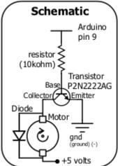
A transistor has 3 terminals. By sending a small current through the **base**, you 'unlock the gate', and a large current can flow from the **collector** to the **emitter**.
